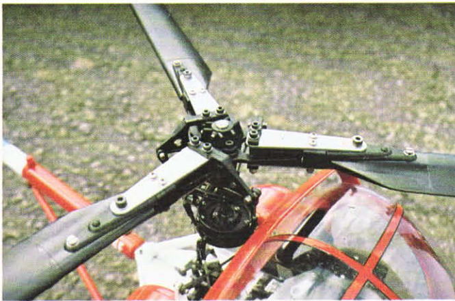
Morley's 3-blade rotor head for the Hughes 300.
