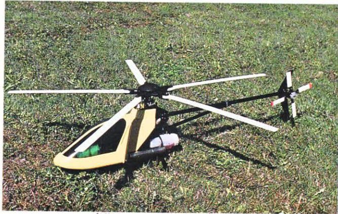
Peka's 5-blade multi rotor head and 4-blade tail rotor on Mark Powelson's Champion which was used as the test bed for testing purposes.
