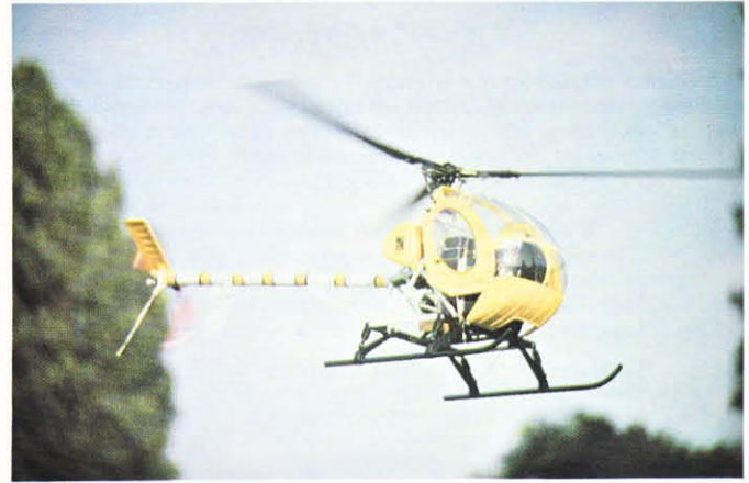
Perfectly controllable and stable, the 3-blade rotor head gives added realism to Morley's Hughes 300.
