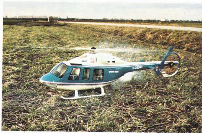
The Twin 400 with the 4-blade elastomeric non bearing rotor head. With either the multi system or elastomeric system the model flies fabulously.
